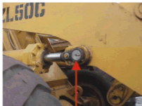
Loadcells installed here
